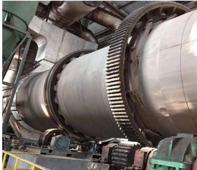
Coal slurry drying set powered by catalytic oxidation system for coal mine gas with methane concentration around 1% to 1.2%.
