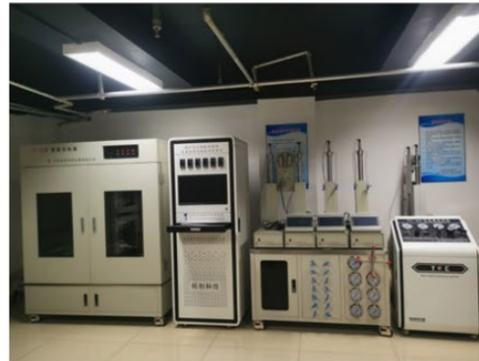
Multi-layered stacked gas reservoir joint development simulator
