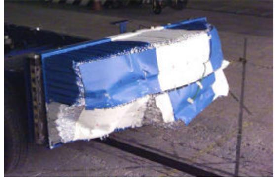
**Figure 12** Cellbond MDB Face, after Vehicle A Test
