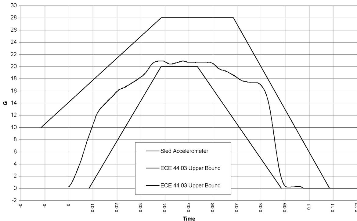
This test was not an isolated case. In fact, the difference in values is even greater when an ECE 44.03 Annex 7 Appendix 2 pulse is analyzed. This is because the pulse falloff is more rapid, so more strain in the system is elastically relieved. Below is the pulse and related data:
