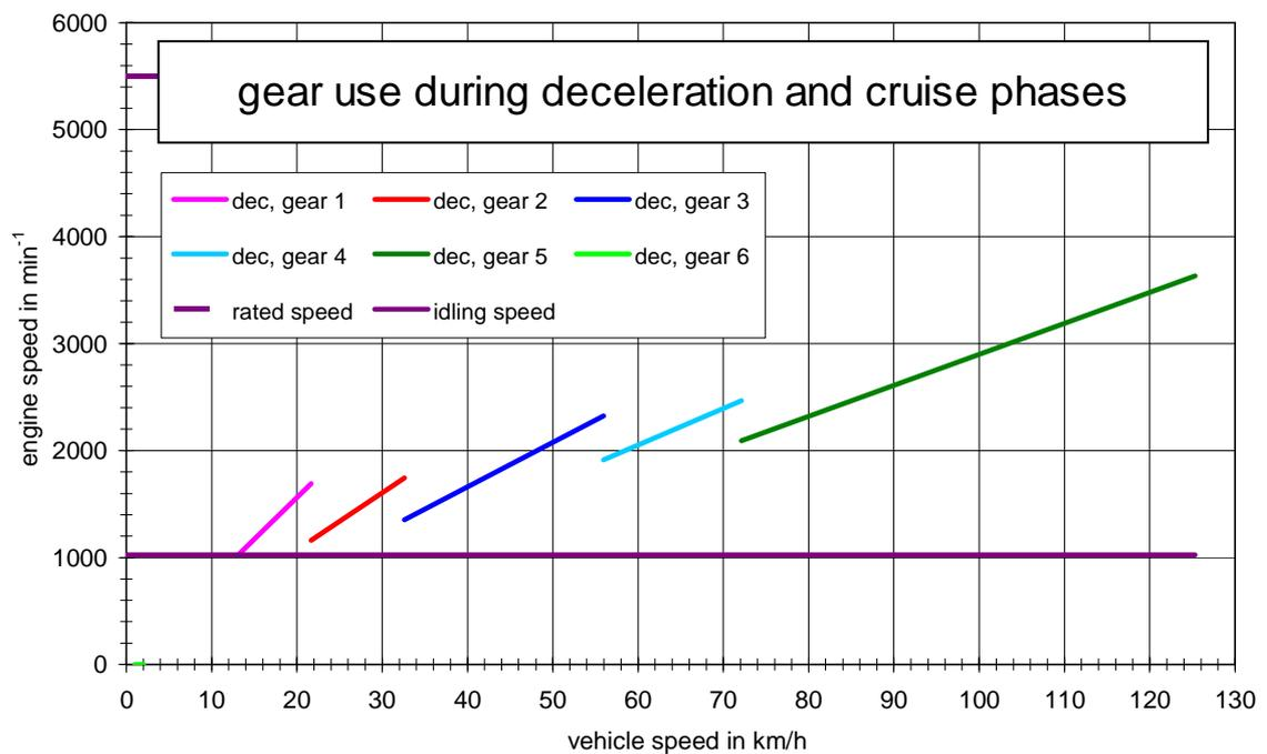
Figure A13-1: Example of a gearshift sketch
