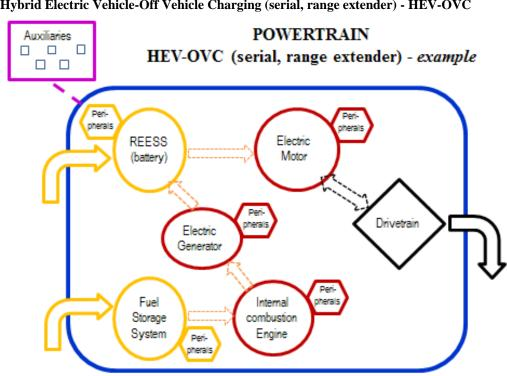
Figure 5 Hybrid Electric Vehicle-Off Vehicle Charging (serial, range extender) - HEV-OVC
