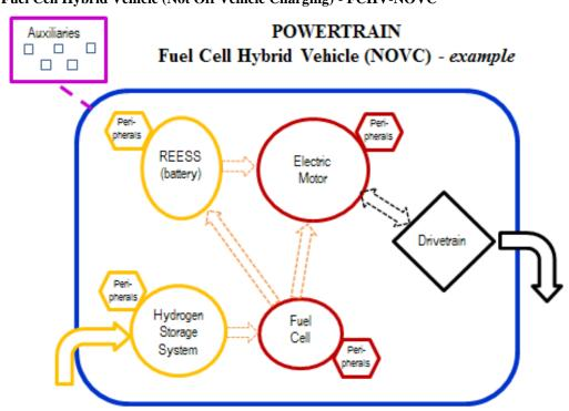
Fuel Cell Hybrid Vehicle (Not Off Vehicle Charging) - FCHV-NOVC
