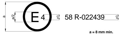
The above approval mark affixed to a vehicle or to an RUPD shows that the vehicle type or RUPD type concerned has, with regard to the rear underrun protection in the event of a collision, been approved in the Netherlands (E 4) pursuant to Regulation No. 58 under approval number 022439. The first two digits of the approval number indicate that the approval was granted in accordance with the requirements of Regulation No. 58 as amended by the 02 series of amendments.
