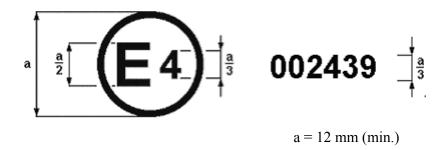
The above approval mark affixed to a pneumatic tyre shows that the type of tyre concerned has been approved in the Netherlands (E 4) under approval number 002439. The first two digits of the approval number indicate that the approval was granted in accordance with the requirements of Regulation No. 54 in its original form.
