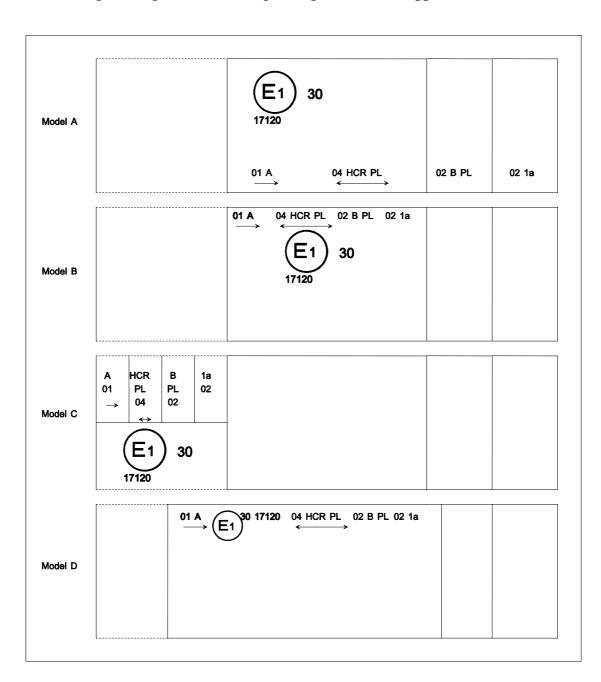
$\underline{\text{Note}}$ : The four examples above correspond to a lighting device bearing an approval mark comprising:
