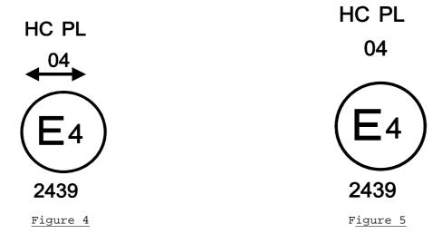
The headlamp bearing the above approval mark is a headlamp incorporating the lens of plastic material meeting the requirements of this Regulation in respect of the passing beam only and is designed:
