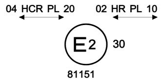
The above example corresponds to the marking of a lens of plastic material used in a unit of two headlamps approved in France (E2) under approval number 81151, consisting of:
