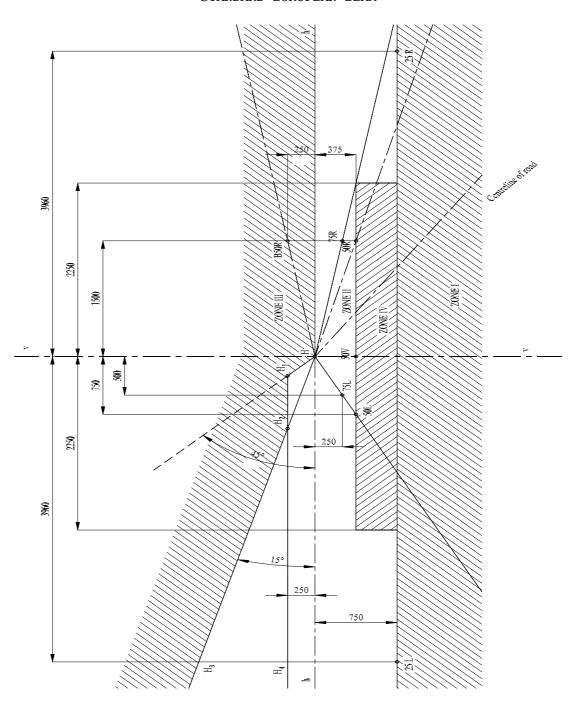
$\begin{array}{lll} \text{h-h} & : & \text{horizontal plane} ) & \text{passing through} \\ \text{v-v} & : & \text{vertical plane} & ) & \text{focus of headlamp} \end{array}$
