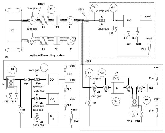
Figure 3 Flow diagram of dilute exhaust gas analysis system for CO, CO<sub>2</sub>, NO<sub>x</sub> and HC
