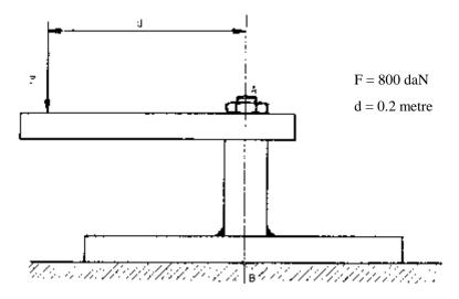
Under a load of 800 daN producing a couple of 160m daN in relation to the point "B", the displacement in any direction of the point "A" shall be lower than 2mm.
