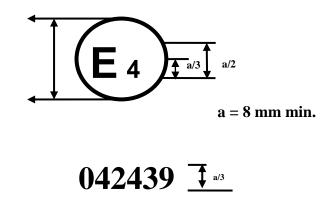
The above approval mark affixed to a steering control shows that the steering control type concerned has, with regard to the protection of the driver against the steering mechanism in the event of impact, been approved in the Netherlands (E4) pursuant to the relevant part of Regulation No. 12 as amended by the 04 series of amendments.
