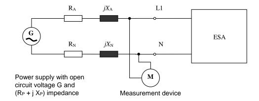
Figure 1b **ESA in configuration "REESS charging mode coupled to the power grid" - Three-phase test set-up** Power supply with open circuit voltage G and  $(R_P + j X_P)$  impedance
