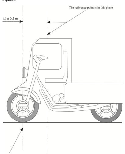
Vertical axis of the front wheel (point C)
