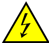
Figure 1 Marking of high voltage equipment
