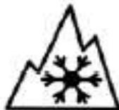
Minimum 15 mm base and 15 mm height when the marking is on the sidewall.
