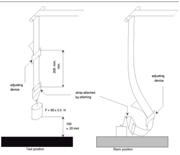
The load of 50 N on the testing device shall be vertically guided in such a way as to prevent load-swing and twisting of the strap. The attaching device shall be fixed to the load of 50 N in the same manner as in the vehicle."
