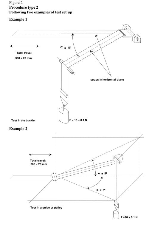
Where  $\alpha$  and  $\beta$  reproduce the angles as in the real installation (in three dimensions).
