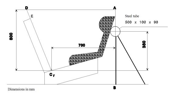
7.1.4.4.1.2.2. Child restraints in group 0 not supported by the dashboard, and carrycots: the head of the manikin shall not pass the planes AB, AD and DE as shown in Figure 3 below. This shall be judged up to 300 ms or the moment that the manikin has come to a definitive standstill whatever occurs first.
