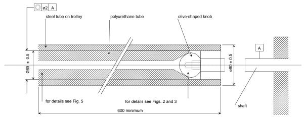
Play defines according to external diameter of the polyurethane tube (light push fit)
