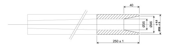
Figure 2 **Stopping device olive-shaped knob**
