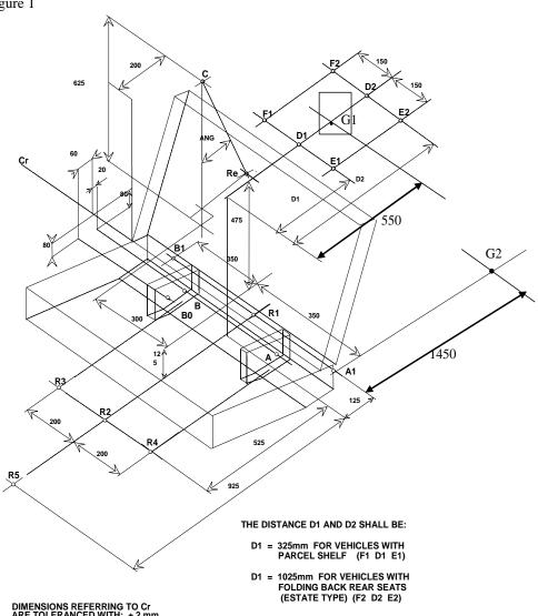
DIMENSIONS REFERRING TO Cr ARE TOLERANCED WITH: ±2 mm EXCEPT FOR DISTANCE FLOOR TO Cr ±10mm
