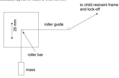
Drop height of mass = 25 mm Distance from roller bar to roller guide = 300 mm Using strap of the webbing specified for the standard seat belt as defined in Annex 13
