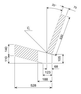
Figure 2 **Dimensions of the aluminium bottom-plate**
