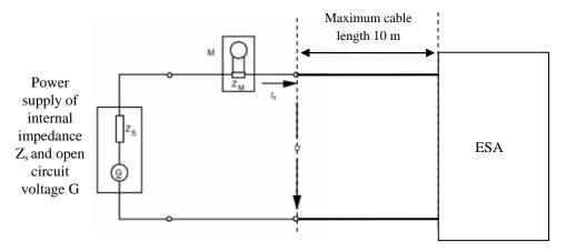
Figure 2 ESA in configuration "REESS charging mode coupled to the power grid" –Three-phase-test set-up
