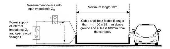
$Figure\ 2 \\ \textbf{Vehicle in configuration ''REESS charging mode coupled to the power grid''-Three-phase charger test set-up}$
