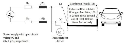
$\label{lem:power_state} \begin{tabular}{ll} Figure~1b \\ \begin{tabular}{ll} Vehicle~in~configuration~"REESS~charging~mode~coupled~to~the~power~grid"-Three~phase~test~set-up \\ \end{tabular}$
