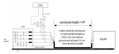
${\bf Figure~4} \\ {\bf ESA~in~configuration~''REESS~charging~mode~coupled~to~the~power~grid''~-~Coupling~between~each~line~and~earth~for~AC~(three~phases)~power~lines}$
