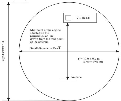
Figure 2 **Position of antenna in relation to the vehicle:**
