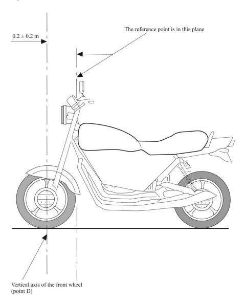
Figure 3 First stage: Determine the reference point Second stage: Rotate the vehicle Rear Front Vehicle-Vehicle Reference point Front Rear Distance maintained between the vehicle and antenna Antenna
