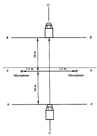
Figure 2 **Positions for testing the stationary vehicle**
