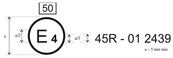
The above approval mark  $\dots$  as amended by the 01 series of amendments. The capacity class is 50.
