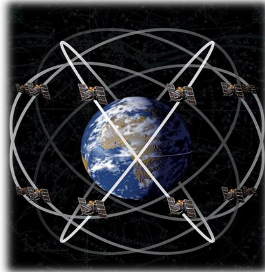
GPS Constellation GPS satellites are positioned in precise, circular orbits 18,000 kilometers (11,000 miles) above the Earth. They orbit once every 12 hours.
