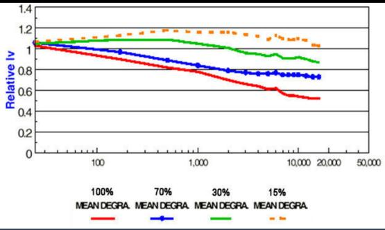
The graphic shows, that only driving the LEDs with less than 15% of their rated current can avoid reduction of light output.
