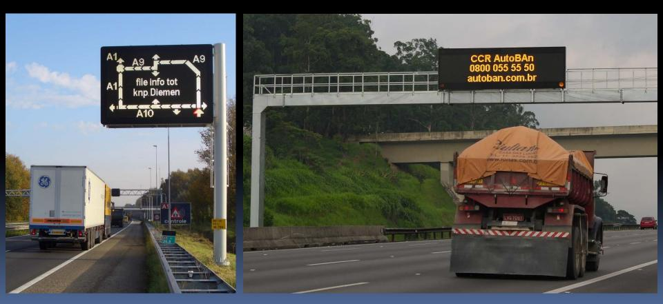
Typical VMS are using different ways for light emitting and reflecting, e.g. LED technology or rotating prisms, used in side tunnels, in hot and cold environment, as parking guidance, as traffic guidance on highways, for toll stations and on many more applications.
