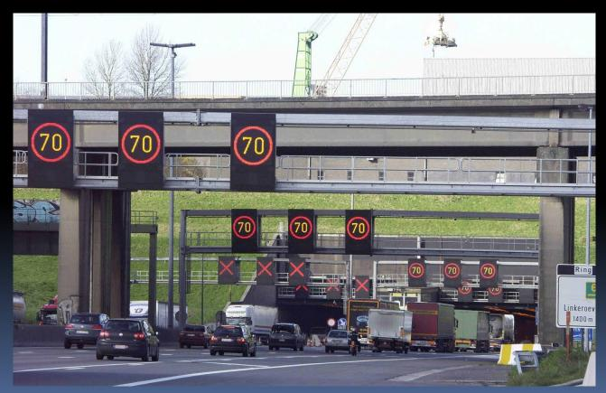
Typical VMS are using different ways for light emitting and reflecting, e.g. LED technology or rotating prisms, used in side tunnels, in hot and cold environment, as parking guidance, as traffic guidance on highways
