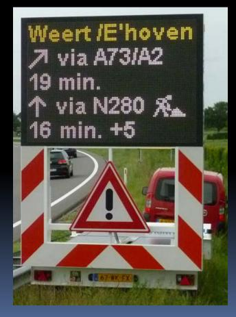
Solar Trailers (Netherlands) 112x8o full graphic RGB (20 mm PP) Display area 3.6 m<sup>2</sup> (38 ft<sup>2</sup>) Control via GPS / GPRS Low-power consumption (av. 68W) 12 signs shipped March '13 Working 20 month only powered by solar energy without recharging Light output (white): 15.000 cd/m<sup>2</sup> Contrast: 27 Beam width: 30°
