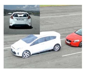
Subject vehicle test speed in test procedures (Para. 6.4, 6.5, 6.6, 6.7)
