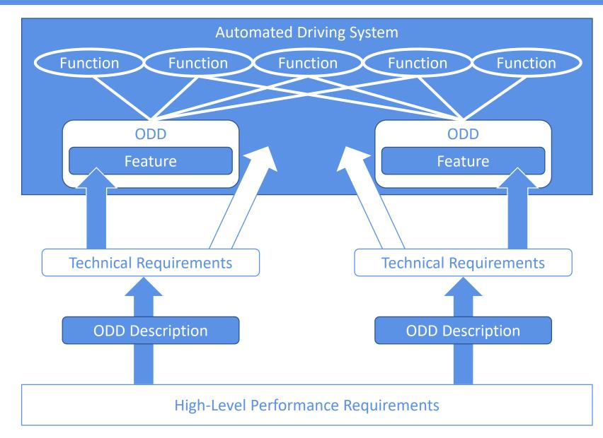
The ADS is the system. An ADS has one or more features. Each feature has a unique ODD. ADS functions perform the DDT. The functions enable the features. Features may use all or some ADS functions and features may share the same functions.
