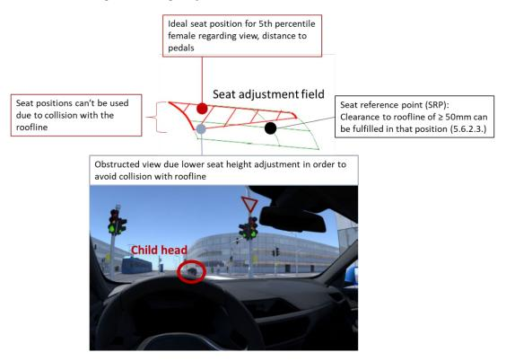
Furthermore a collision with the roof may have an impact to the easy-entry function for 2-doors vehicles with more than one seat row and to the curtain airbag deployment.
