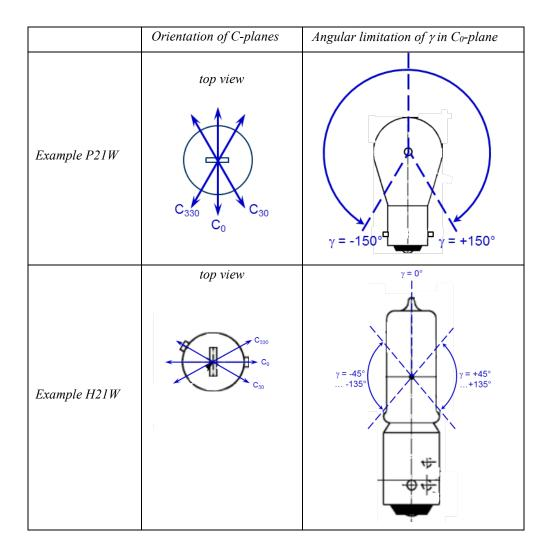
Figure 1: representative examples of filament positions and limitations of the directions where light emission of the LED replacement light source should be specified
