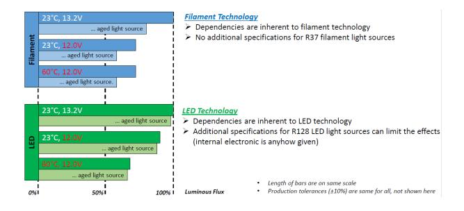
Figure 10: Comparison of filament and LED technology with respect to the voltage- and temperature-dependency of the luminous flux (incl. ageing)
