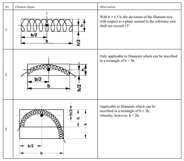
The side lines of the circumscribed rectangles in Nos. 2 and 3 are parallel and perpendicular, respectively, to the reference axis.
