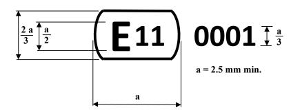
The approval mark above affixed to a filament-light source indicates that the light source has been approved in the United Kingdom (E 11) under the approval code 0001.
