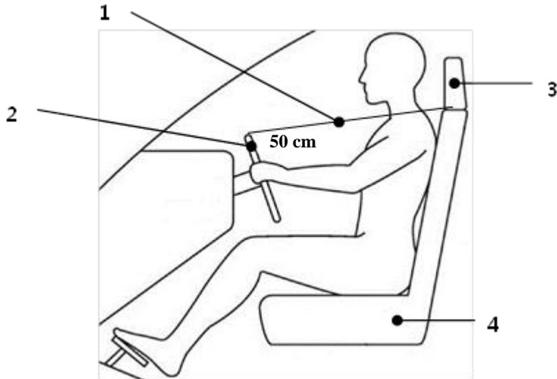
1. Vehicle Sampling Point Location, 50 centimeters from top of steering wheel to bottom of headrest.
