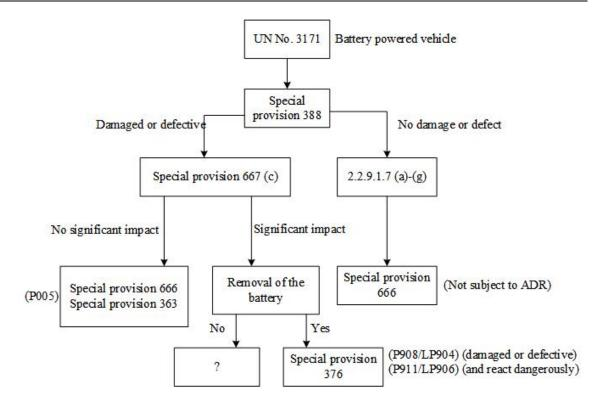
2. The danger is recognized, but there are no regulations on transport or packaging for damaged electric vehicles. Damaged or defective lithium batteries can heat up and start to burn. It does not matter whether the batteries are still installed on the electric vehicle or not. Precautions must be taken and any such situation brought under control as quickly as possible.
