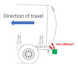
3. The current text of 9.7.6 (ADR 2019) requires "a clearance of at least 100mm between the rear wall of the tank and the rear of the bumper (this clearance being measured from the rearmost point of the tank wall or from projecting fittings or accessories in contact with the substance being carried)." It would therefore seem that the intention is as follows:
