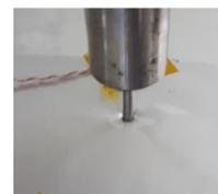
**Figure 6 : Nail penetration test of a fully charged pouch cell**
