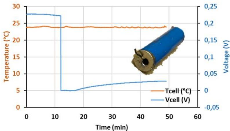
Figure 10: Nail penetration test result for a fully discharged 18650 cell
