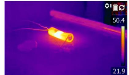
**Figure 5: Crush test result for a fully charged 18650 cell**
