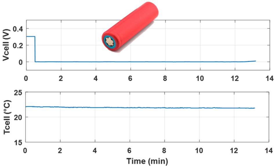
Figure 8 : External short-circuit test result for a fully discharged cell
