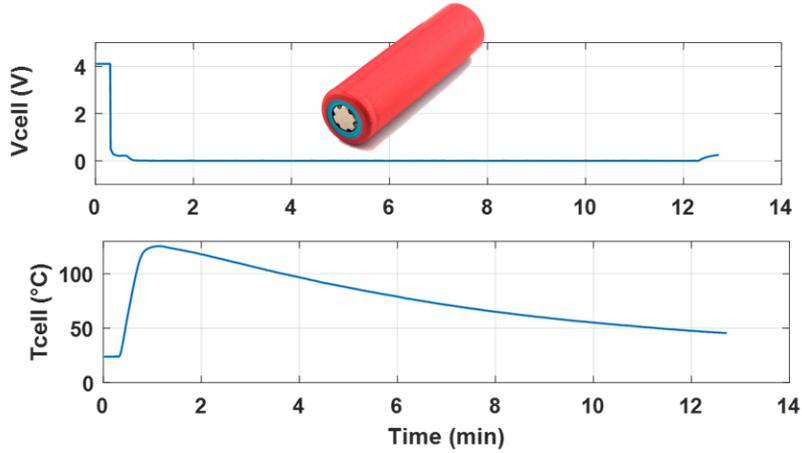
Figure 3 : External short-circuit test result for a fully charged cell
