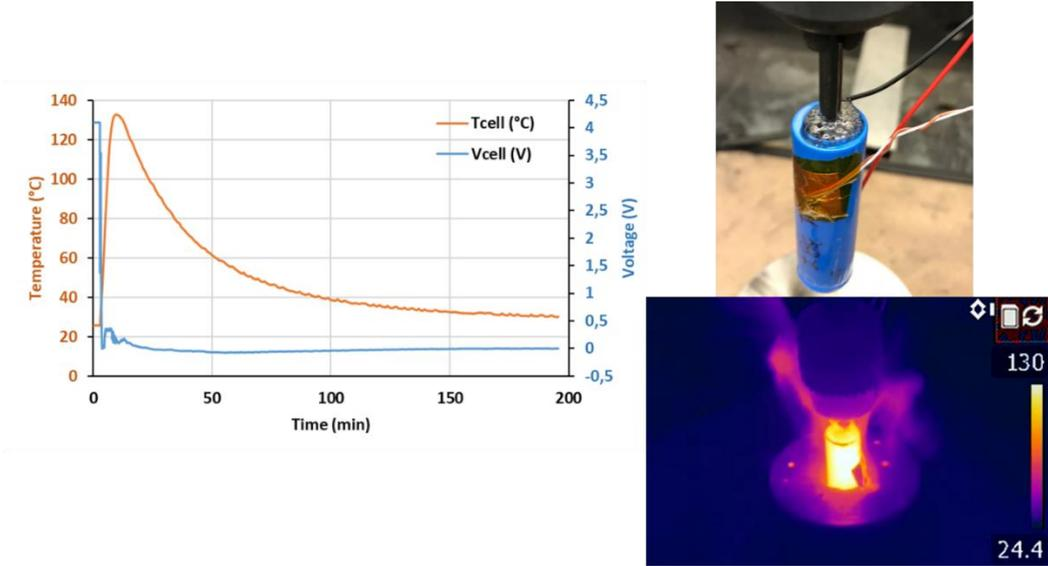
Figure 7: Nail penetration test result for a fully charged 18650 cell
