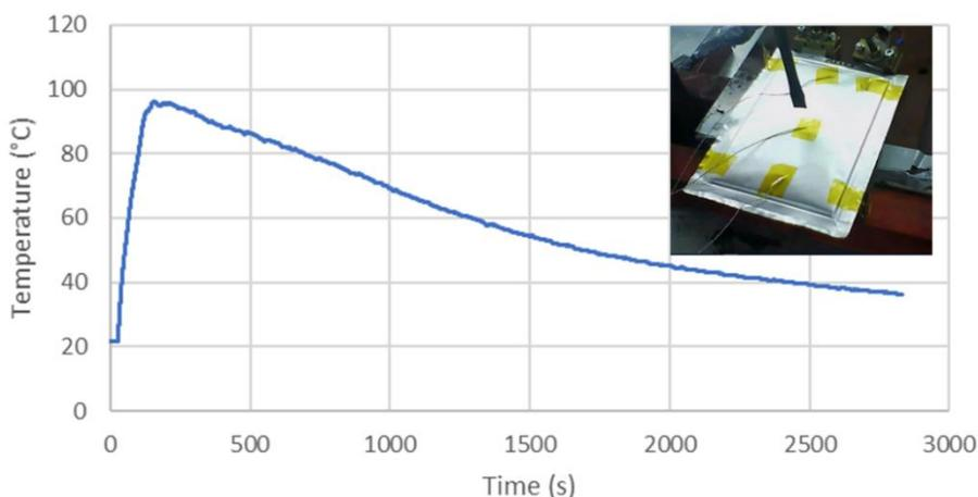
**Figure 2 : External short circuit test of a fully charged pouch cell**
