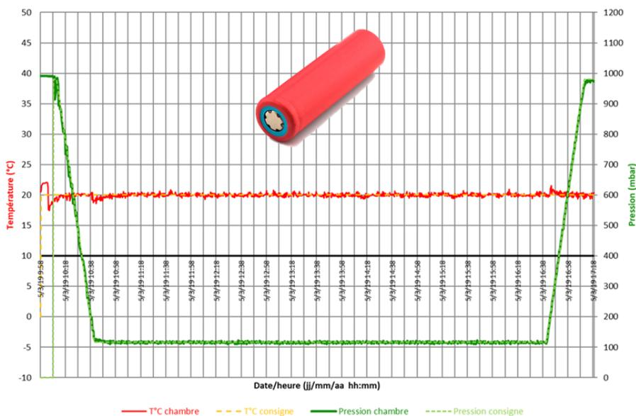
**Figure 1 : Altitude simulation test result for fully charged 18650 cells**
