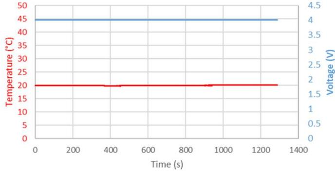
Figure 4 : crush test of a fully charged pouch cell
