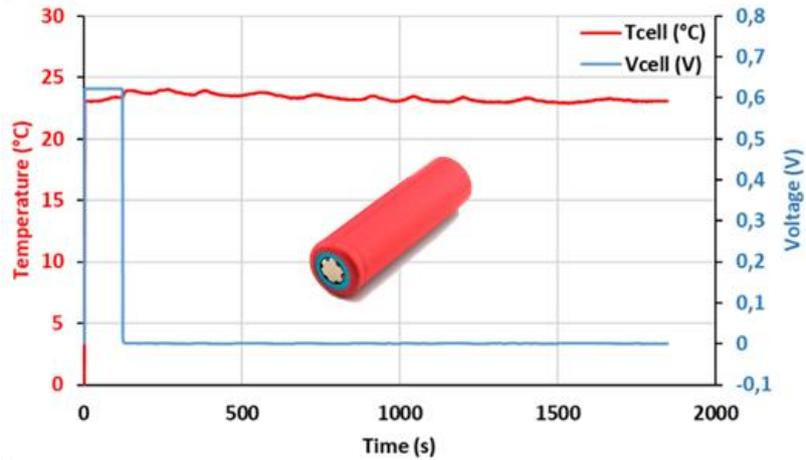
Figure 9: Crush test result for a fully discharged 18650 cell
