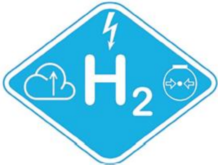
Example of label for Fuel Cell Electric Vehicle container holding compressed gas which is lighter than air
