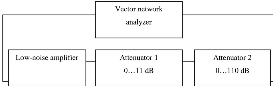
2.7.3. Set zero signal path attenuation on attenuators. Measure the frequency response for a given signal path in the L1/E1 band of GNSS GLONASS/Galileo/GPS. Record the average path transmission factor in [dB] in this frequency band.
