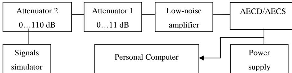
2.7.5. Prepare and turn on AECD/AECS according to operational manual. By means of developer software make sure that GNSS receiver is set to receive GNSS GLONASS, Galileo and GPS signals. Clear the navigation module RAM<sup>2</sup> such that the "cold" start mode of the navigation module of the AECD/AECS is achieved. Check that the position, velocity and time information is reset.
