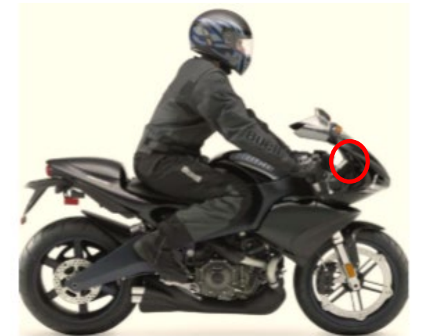
Motorcycle with Cockpit and Windscreen – Instruments Directly Face the Rider (sensor therefore in shadow)
