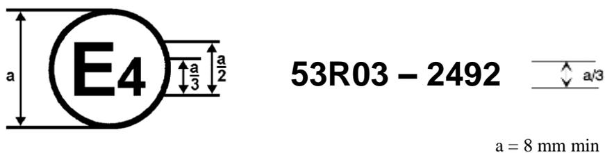
The above approval mark affixed to a motorcycle shows that the vehicle type concerned has, with regard to the installation of lighting and light-signalling devices, been approved in the Netherlands (E 4), pursuant to UN Regulation No. 53, as amended by the 03 series of amendments. The approval number indicates that the approval was granted in accordance with the requirements of UN Regulation No. 53.
