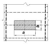
Dimensions of the loading platform, m, when vehicles move along the beam framing (see fig. 10.6.1.8-1 and fig. 10.6.1.8-2) are determined by formulas:
