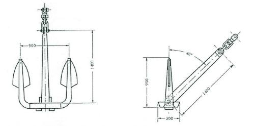
A tolerance of  $\pm 5\%$  applies to the dimensions and mass given. However, the surface area of each fluke must be at least 0,15 m<sup>2</sup>.
