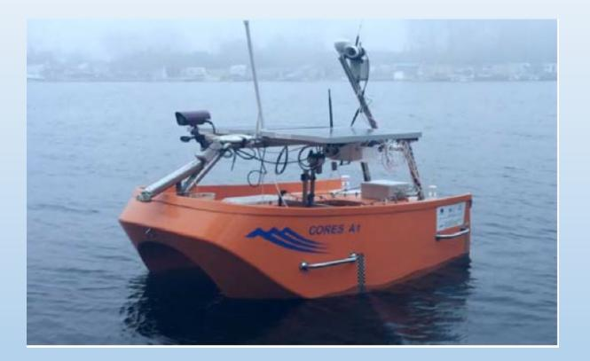
Zero-emissions Solar Powered USV Boat for Hydrographyc Survey
