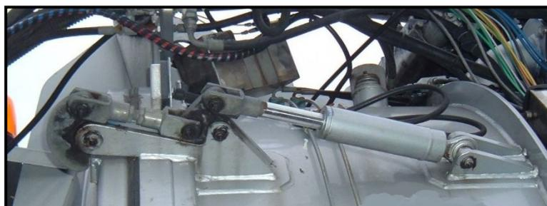
The paper advises that these types of door clamping mechanisms would appear to be vulnerable to damage that could allow the door to be forced open in the event of a roll-over incident and therefore, in our opinion, such design would not seem to meet the requirements of ADR 6.10.3.5 (e) unless additional measures were to be put in place to protect the locking mechanism.
