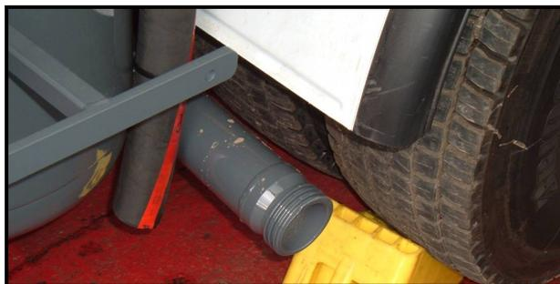
The hose will be connected to either (a) an on-site device that cleans the output from the vacuum pump or (b) an extension hose that is approximately 15m long and allows the vapours to be vented in a safe place (i.e. away from potential hazards, sources of ignition and personnel).
