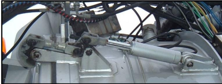
6. In our opinion the examples shown in (a) and (b) above would seem to meet the requirements of 6.10.3.5 (e). In respect to example (c) however, given the door clamping mechanism would appear to be vulnerable to damage and allow the door to be forced open in the event of a roll-over incident, in our view this design would not seem to meet the requirements of 6.10.3.5 (e) unless additional measures were to be put in place to protect the locking mechanism.
