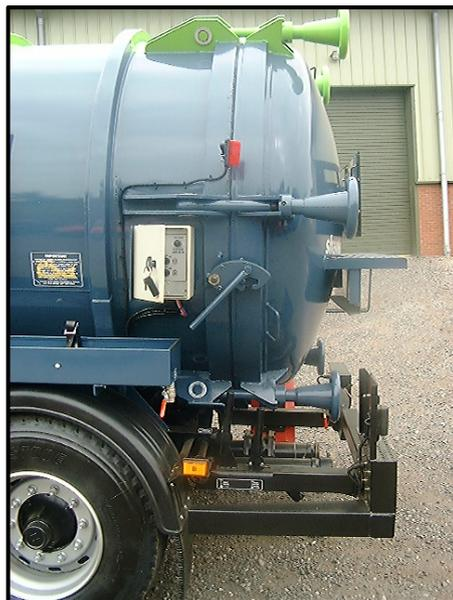
It should be noted that, as required by ADR 6.10.3.5 (d), the above locking arrangement incorporates a safety device to prevent the door opening when there is still residual pressure in the tank.
