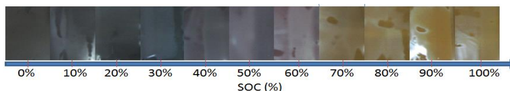
Figure I: Effect of state of charge (SOC) on lithium ion intercalation state
