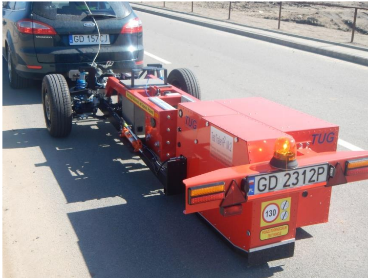
Figure 1 The TU Gdansk measurement trailer for measuring rolling resistance on road surfaces.
