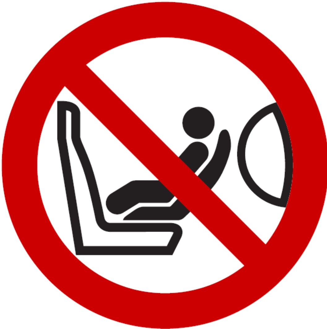
Figure B Pictogram according to ISO 2575:2004 - Z.01 that shall be used and that shall have an outer diameter of at least 38 mm
