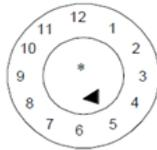
\* The last two digits of the year of manufacture may be displayed at that place. In this case and under condition the clock is placed adjacent to UN design type mark, the indication of the year in the type approval mark may be waived. However, in case the clock is not placed adjacent to the UN design type mark, ~~In such a case,~~ the two digits of the year in the ~~type approval~~ mark and in the ~~inner circle~~ of the clock ~~should~~ shall be identical.
