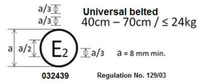
The Enhanced Child Restraint System bearing the above approval mark is a device capable of being fitted in any universal seating position of the vehicle and of being
