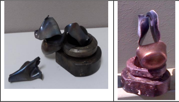
“E”: Tube split into two fragments
