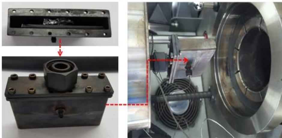
Fig.5 it shows a sequence of installing a cell in an ARC chamber. In the left side a tube is seen, including a pouch cell whose tabs were cut, and in the right side a picture is showing before the tube is put into the electric furnace of ARC equipment (TIAX). In order to raise objectivity in the ARC tests, all tasks including cell formation were executed at and through TÜVSÜD Korea (<http://www.tuv-sud.kr/>).
