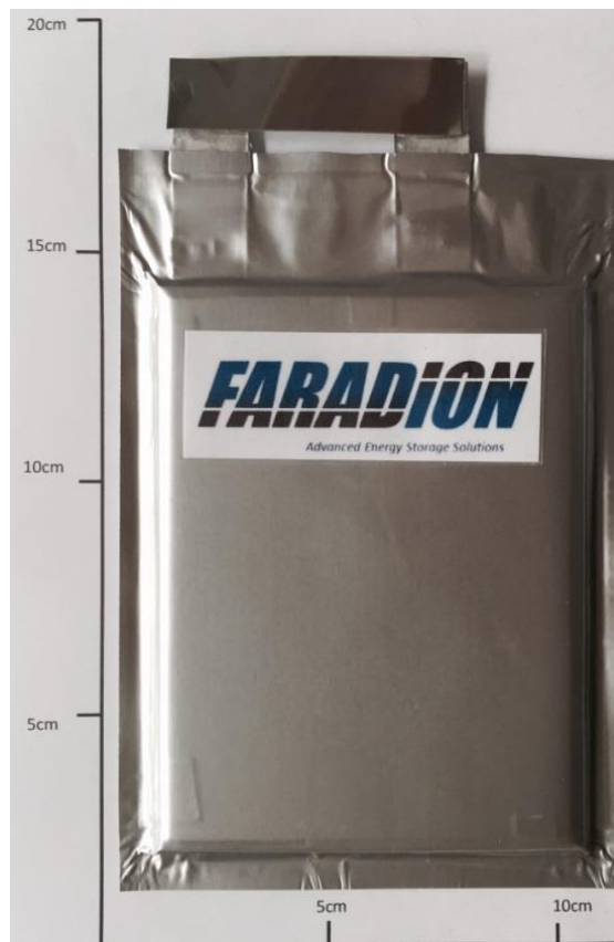
Figure 8: Example of a sodium-ion battery cell which is shorted between the positive and negative terminals and displays visual verification of the short from the metallic strip connecting the terminals
