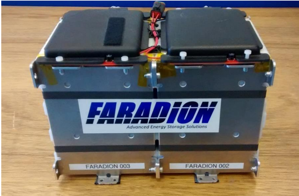
Figure 7: Sodium-ion battery comprised of two modules, each containing twelve 13 Ah cells.
