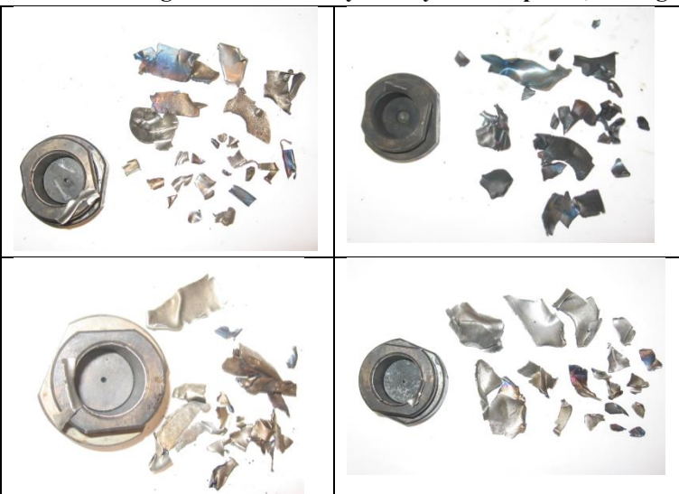
“G”: Tube fragmented into many mainly smaller pieces, closing device undamaged
