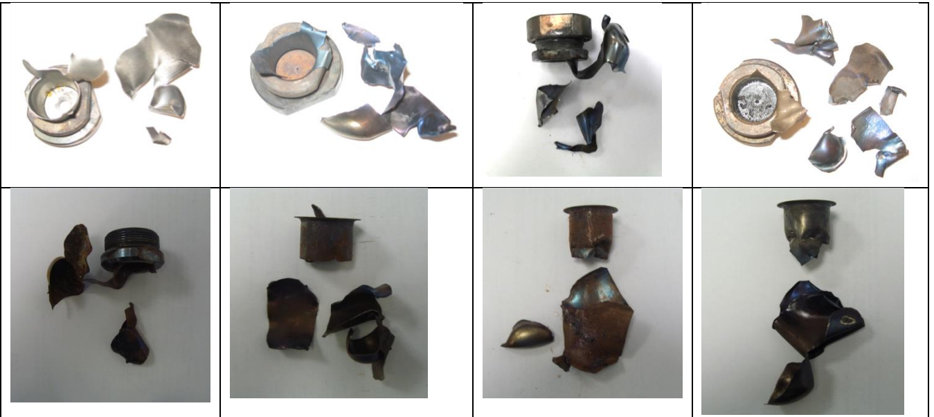
“F”: Tube fragmented into three or more mainly large pieces which in some cases may be connected with each other by a narrow strip;
