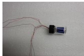
**Figure 6: Metal-free detonative initiator**
