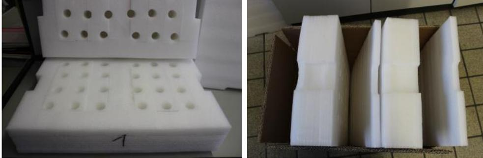
**Figure 7: Foam matrix for sample containers**
