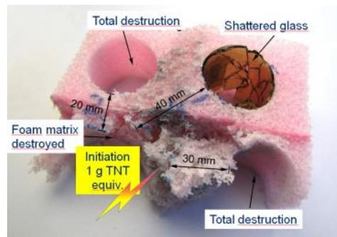
**Figure 8: Propagation of detonation at different distances**
