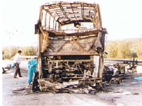
Fig.10. Fire after frontal collision
